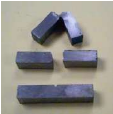
Figure 18 Ductile Fracture (top) Brittle Fracture (centre) Initial Specimen (bottom)
