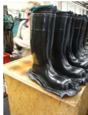
Figure 45 Car Tyres and other rubber products are manufactured using compression moulding
