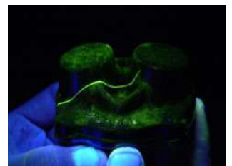
Figure 7 UV Liquid Penetrant Test
