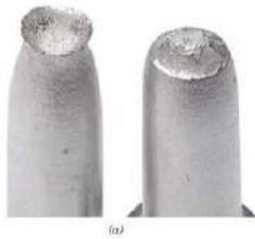
Figure 22 'Cup and Cone' Fracture
